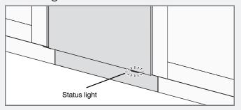
The status light at the bottom of the dishwasher provides information by means of 3 different colours.
