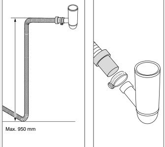
The drainage hose can also be connected to a connection nipple on the sink unit's water trap. The connection nipple must have an internal diameter of at least 14 mm.
