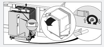
4 Adjust the front feet by turning them clockwise to raise and anticlockwise to lower the dishwasher.
