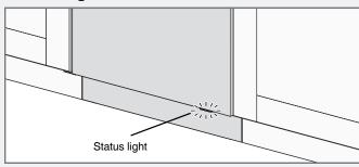
The status light at the bottom of the dishwasher provides information by means of 3 different colours.
