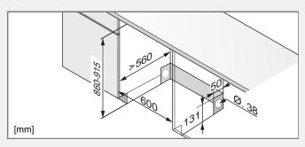
If the dishwasher is built-in the surrounding cabinetry must be resistant to any condensation from the dishwasher.
