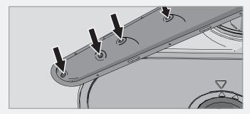
To facilitate cleaning, you can remove the spray arms. Remember to fit them firmly back into place after cleaning.
