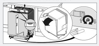
4 Adjust the front feet by turning them clockwise to raise and anticlockwise to lower the dishwasher.
