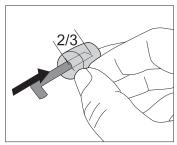
4 - o- If the filter foam is detached from the inlet pipe, replace it by inserting the pipe to the depth of two thirds of the overall foam length.
