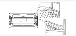
With telescopic extendible guides, first pull out the guides of one level and place the grid or the baking tray onto them. Then, push them in with your hand as far as they will go.
