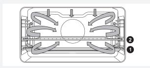
When grilling directly on the grid, smear it with oil to prevent the meat from sticking onto it and insert it into the 2nd guide. Insert a drip tray into the 1st guide. When roasting meat in a baking tray, insert it into the 1st guide.
