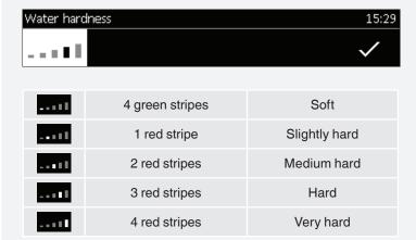
Soak the test paper strip (supplied with the appliance) in water for one (1) second.
