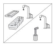
Clean the inlet pipe with the filter foam under running water. Rinse the foam clean so that there are no visible impurities on it. Thus, you will make sure the appliance operates correctly and preserve the fresh flavour and smell of food.
