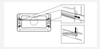
**BAKING PAN SUPPORT** allows easy removal of baking pans from the oven while they are still hot.
