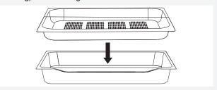
In case of wire guides, the tray should always be inserted into the groove between the two wire profiles.
