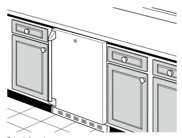
Cut-out dimensions: Height: 877 mm minimum
